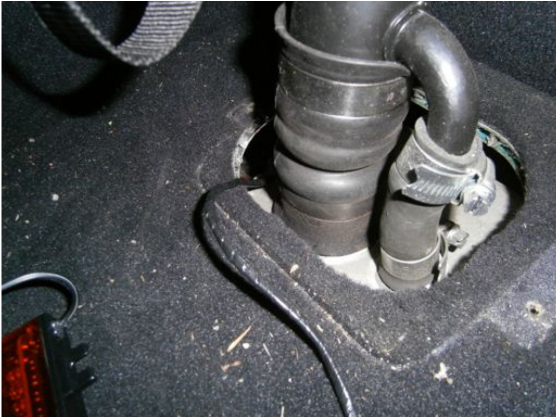
fig4 - Caterham high-level sub-loom through the RHS of fuel filler hole
