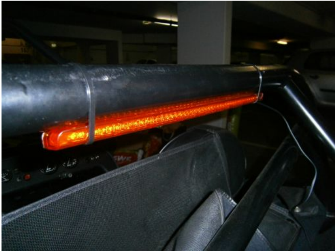
fig7 - 48-LED lights cable tied to underside of rollbar
